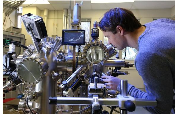
Image: Researcher, Joris Keizer, using a scanning tunnelling microscope to fabricate silicon devices with atomic precision
